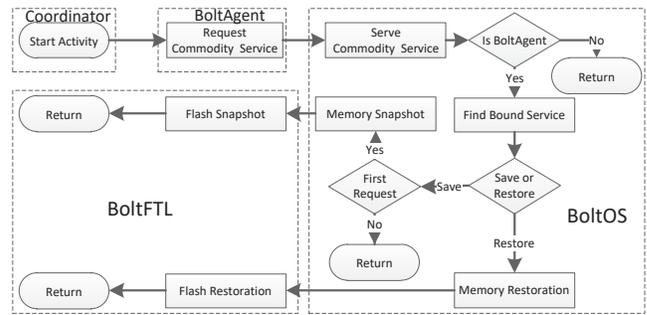
**Figure 3: Bolt work-flow.**
