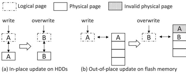
**Figure 1: Comparison of an overwrite operation between HDD and flash memory.**
